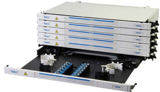
Figure 1: A standard 4 RU/6-tray panel. With 24 ports per tray, total panel capacity is 144 terminations.
