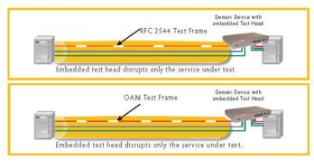
Embedded test head using industry standards (MEF, IEEE and ITU) enables non-disruptive test for frame delay, frame delay variation and throughput
